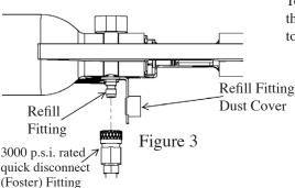
To refill your Spin-Loc Tank, attach the 3000 p.s.i. rated quick disconnect to the refill fitting. See FIGURE 3.
