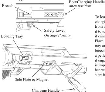
To load the rifle, pull the charging handle away from the frame and push it toward the muzzle until it cannot open any further. Place a pellet in the loading tray and push it into the breech, with your thumb or a pellet seating tool, until it engages the rifling. This is important for accuracy, because it makes each shot start from the same place.
