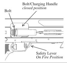
⚠ WARNING: Do not move the safety to the On Fire position unless the air gun is pointed in a safe direction. Safe means that if the gun discharged it would not cause injury or property damage. Mechanical safeties are not infallible and do not replace the need for responsible gun handling practices.
