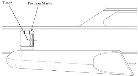
To increase tuner tension rotate it downwards, to decrease tension rotate it upwards. Increasing tension can help achieve higher velocities for light-weight pellets.
